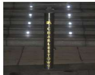
Decorative Fixed Bollards- galvanised and stove enamelled Fixed c/w base plates- 1mH- Unit cost = c. €275.00
